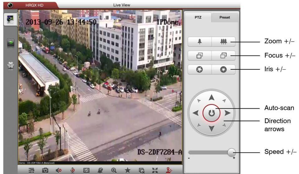
Use the PTZ controls to adjust the PTZ speed, pan/tilt movement, iris, focus, and zoom.
