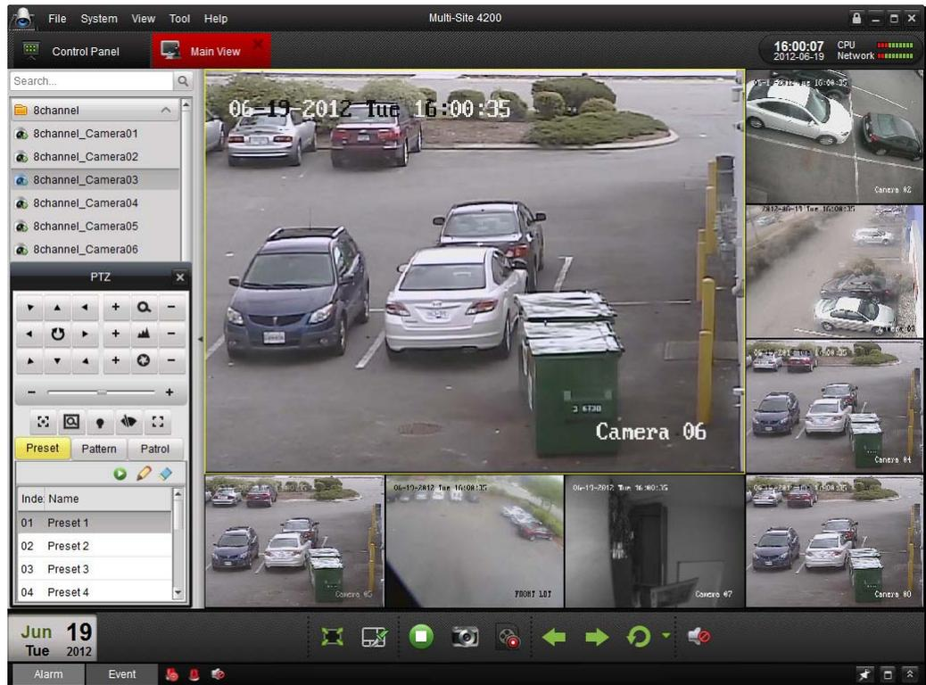
Click on those directional buttons to control the PTZ function (see [Figure 3-23](#)). You can also control the PTZ direction by the directional buttons on your keyboard.
